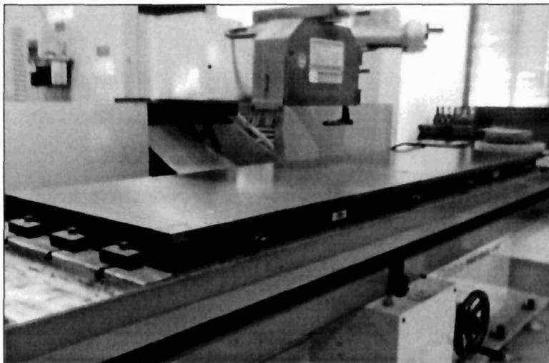
Figure 2.1: Gate Precision Surface Grinding Machine
