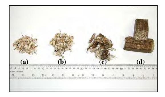
Figure 2.3: Core fiber material; (a) small, (b) medium, (c) large and (d) compresses into a square cube.
