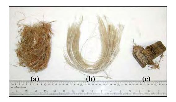
Figure 2.2: Bast fiber material; (a) Kenaf bast fiber strands while fiber strands after harvesting with a forage chopper, (b) retted combed fiber strands and (c) fiber strands compressed into a square cube.
