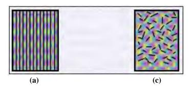
Figure 2.8: (a) Continuous fiber composites and (b) short fiber composites
