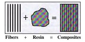
Figure 2.7: Formation of a composite material using fibers and resin.
